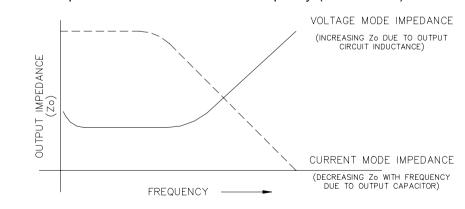
FIGURE 2-4. VARIATION OF OUTPUT IMPEDANCE WITH FREQUENCY FOR A VOLTAGE SOURCE AND A CURRENT SOURCE
