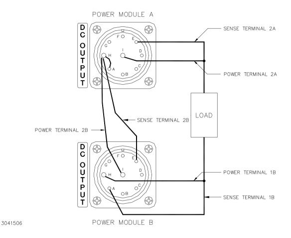
FIGURE 3-1. TWO MAT 1/3 RACK POWER MODULES CONNECTED IN SERIES VIA THEIR OUTPUT CONNECTOR
