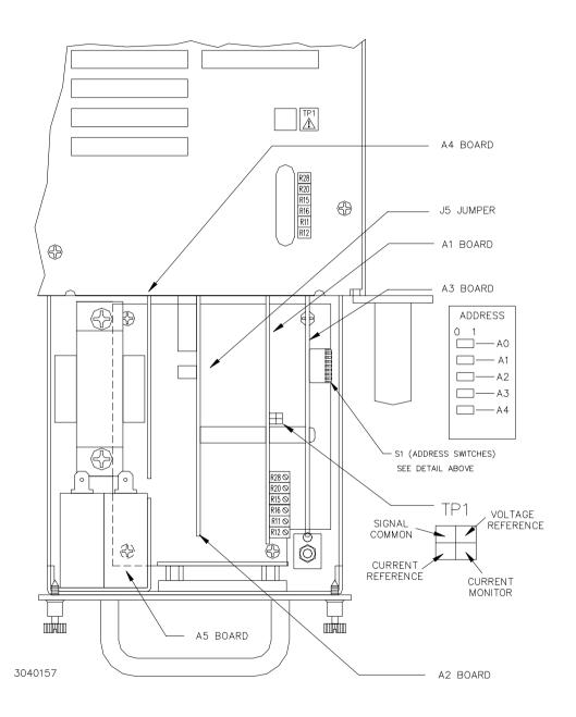
FIGURE 3-2. MATPOWER MODULE CONTROL SECTION, TOP COVER REMOVED
