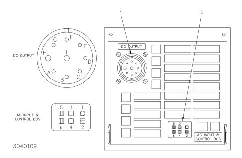
FIGURE 2-2. REAR VIEW OF THE 1/3 RACK POWER MODULE
