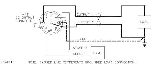
FIGURE 2-5. LOAD CONNECTIONS, LOCAL SENSING
